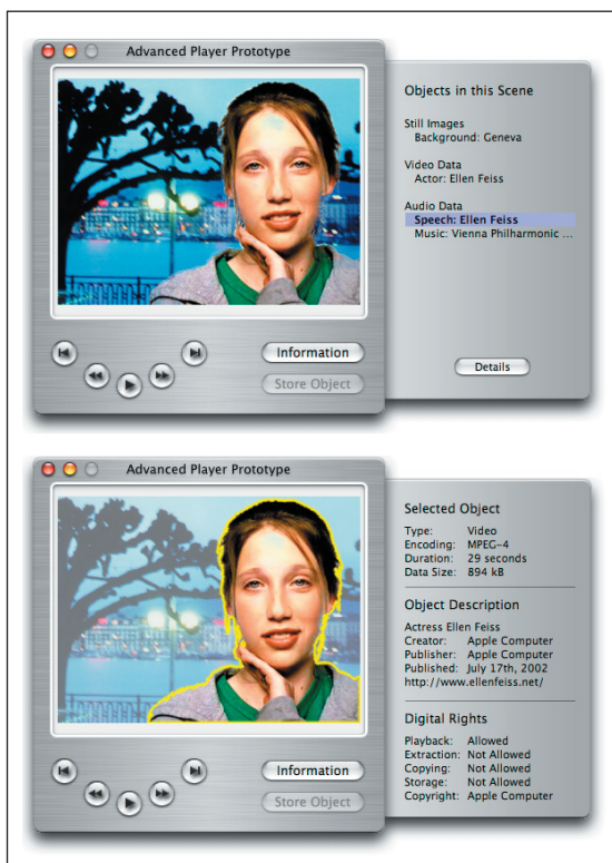
Figure 3: Prototype user interface of a player application for Vivid. Top: if no object is selected and the user presses the "Information" button, a list of object in the scene is shown. Bottom: information about a particular object (the actress) of the displayed content. The picture of Ellen Feiss was taken from [Feiss 2002].
